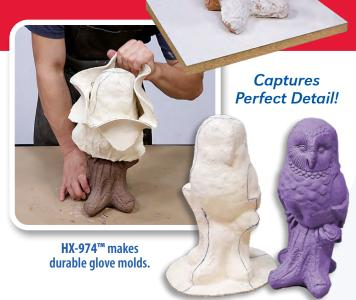
The HX-974™ mold is used to make a casting.
