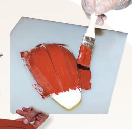
Ultratough **EpoxAcoat™ RED** tool is ready to make composite parts for motorcycles.
