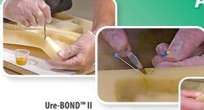
Ure-BOND™ II is being used to repair a tear in a urethane mold.
