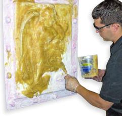
Plasti-Paste™ II holds a vertical surface without sagging for making lightweight mother molds.
