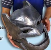
Cast Magic™ Pig Iron and Smooth-Cast™ ONYX™ resin are used to create a luster and shine similar to real metal.
