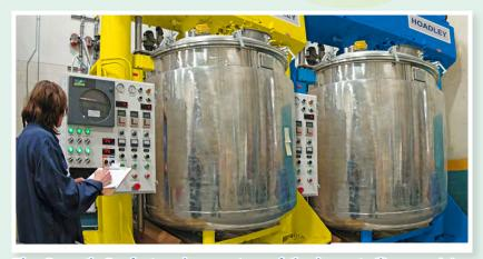
The Smooth-On factory houses two of the largest silicone mixing vessels in North America (1,500 gallons/5,678 liters), each powered by  $3 \times 100$  horsepower motors and high-shear mixing blades.
