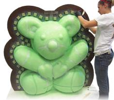
**EZ-Brush™ Vac Bag** silicone can also be used for fast, large scale brush-on molds.
