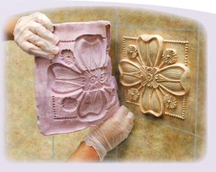
**Equinox™** silicone putty is perfect for making molds on-site when other methods can't be used.
