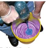
Turbine Mixer has a simple design, yet does a better job of mixing rubbers, plastics, and foams than any mixer we've tried. It also mixes powder-based Alja-Safe™ alginate and Matrix™ NEO with fiber better, and is easy to clean.
