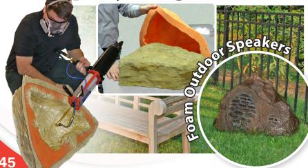
**EZ~Spray™ Rigid** and **Flexible Foams** are a polyurethane foam compound that can be conveniently sprayed using Smooth-On's **EZ~Spray™ Jr.** spray system.
