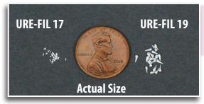
**URE-FIL™ 17** are small grain aluminum pellets (400 micron). Smaller grain pellets will settle into areas of detail better, reducing voids between particles.
