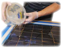
**Solaris™** is a low viscosity, clear silicone designed to protect electronic components and other assemblies against shock, vibration, moisture, ozone, dust, chemicals and other environmental hazards. The optical clarity of **Solaris™** makes it suitable for potting solar cells for maximum light transmission or electronic assemblies where component identification is necessary.
