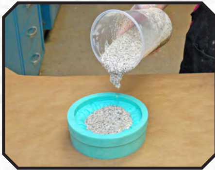
2. After thoroughly combined, pour mixture into mold.
