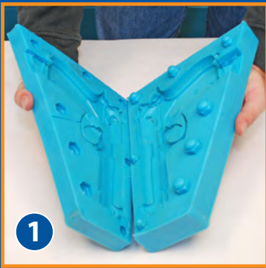
1. A two-piece Mold Star ® silicone mold is used for casting TASK ® 16.
