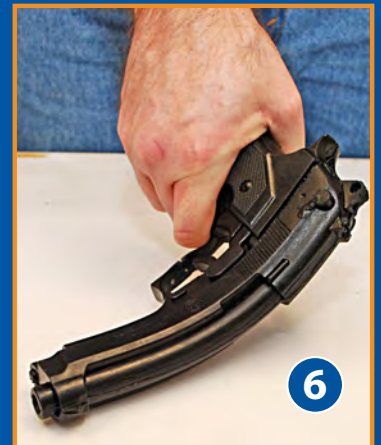
6. Prop Gun is very realistic looking and durable. Castings will flex slightly and are highly impact resistant.
