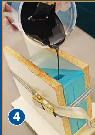
4. Tinted resin is poured into the mold and allowed to cure for 90 minutes.
