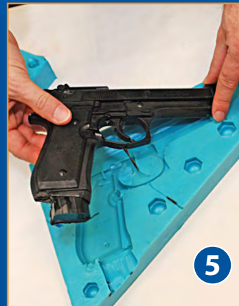
5. Finished TASK ® 16 prop gun casting is demolded and displays incredible detail.
